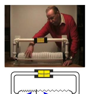
And like it is shown in the left figure I have constructed a closed loop with a tube and a bellow, the latter centrally subdivided by a plate, with which I can create a push-pull flow in the tube, while in the upper branch of the tube locally a flexible yellow membrane is mounted in the wall, which registers what happens on the wall of the tube.
