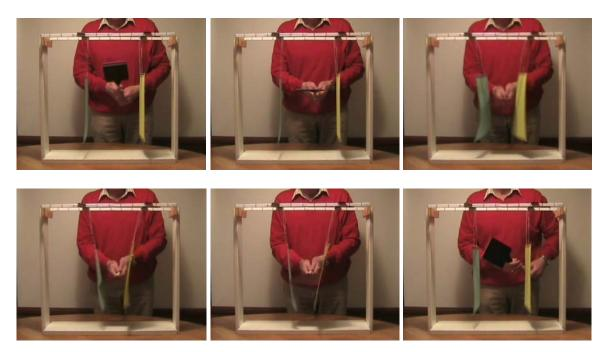
The tube experiment also shows that the membrane in the wall is always moving inwards – so towards the core line of the tube. And superposed on a constant deflection inwards the membrane also deflects periodically with double frequency related to the original stimulus frequency.
